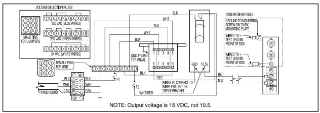
Figure 2. WLVEH Outdoor Enclosure Wiring Diagram
